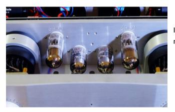
Insert the tubes in the correct position, as marked.
