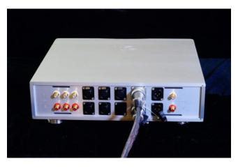
Connect the two cables between the Power Supply and the Amplifier section. Connect the cable to Plug A on both units and the second cable to Plug B on both units. There are several guides on the plugs; one is much thicker than the others. The thick guide is always to the top of the plug.
