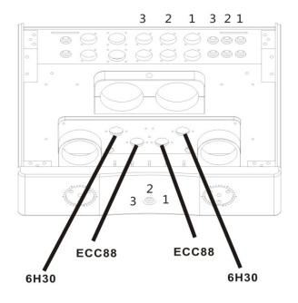
Ensure that the tubes are inserted as per the diagram.
