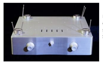
Place the chassis on a firm surface upside down, and remove the eight screws as shown in the diagram. A Phillips Head Screwdriver will be required.
