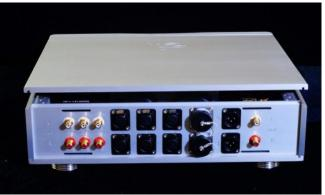
Hold the top in place whist you turn the unit over onto its feet, and carefully remove the top plate which is surprisingly heavy.
